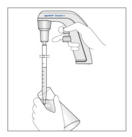
To dispense the liquid, hold the disposable serological pipette vertically and place it on the tube inner wall. Begin by pressing the dispensing control button to allow the liquid to flow (slow dispensing) or blow (fast dispensing) out. During the blow-out the liquid will be dispensed using the pump. When complete, discard the disposable serological pipette into the yellow coloured waste bin/container.
