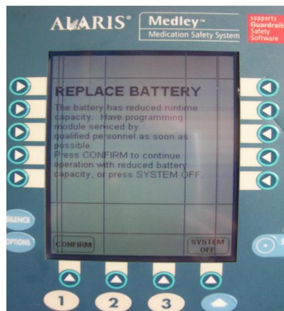
**Defective Battery** – pressing the silence key will allow temporary operation, the pump should be sent to Clinical Engineering immediately.
